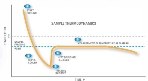
Advanced<sup>®</sup> osmometers utilize the industry-preferred freezing point depression method to determine the osmolality of an aqueous-based solution. When a solute (particles) is dissolved in a solvent (water), the freezing point of that solution is lowered compared to that of the solvent alone. As more solute is added, the freezing point decreases further. Therefore, by precisely measuring the freezing point of the solution, the osmolality (i.e., concentration) can be determined.
