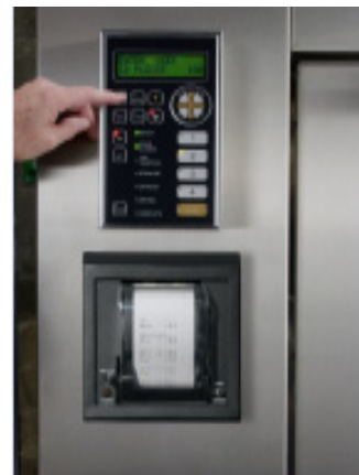
Standard Control Panel /Printer Arrangement
